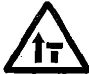
Lane closed (Two Lane road)
